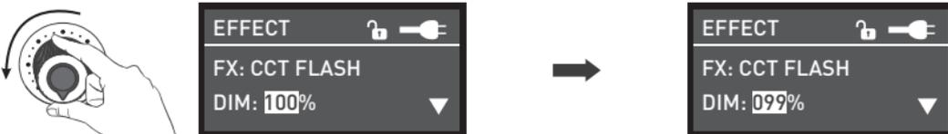
Rotate the "left knob" to set the parameters of the corresponding options.
