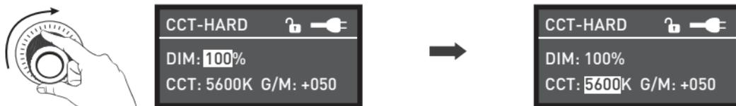
Rotate the "right knob" to select DIM, CCT and G/M.
