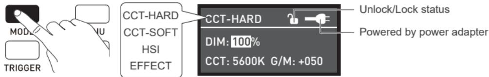
① CCT-HARD mode, rotate the "right knob" to select DIM, CCT and G/M, rotate the "left knob" to set the parameters of the corresponding options. DIM range: 000%...100%, CCT range: 2700K... 7500K, G/M range: -100...+100.
