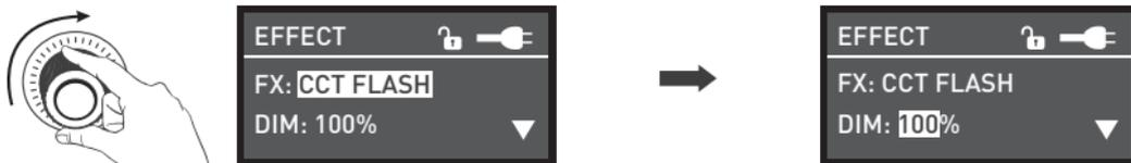
Rotate the "right knob" to select DIM, CCT, G/M and INTVL.
