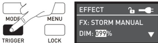
Press the TRIGGER button to trigger the STORM MANUAL effect.
