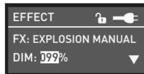
Rotate the "left knob" to set the parameters of the corresponding options.
