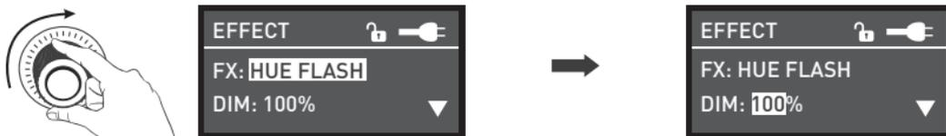
Rotate the "right knob" to select from DIM, HUE, SAT and INTVL.
