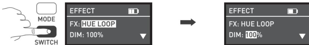
Press SWITCH button to select from DIM, HUE and SPD.
