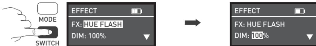
Press SWITCH button to select from DIM, HUE, SAT and INTVL.
