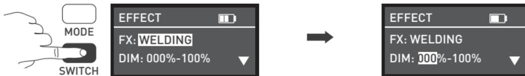
Press SWITCH button to select from DIM, CCT, G/M, SPD and PAUSE.
