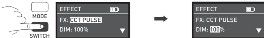
Press SWITCH button to select from DIM, CCT, G/M and PULSES/M.
