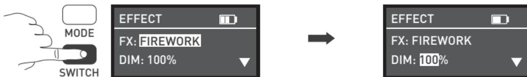
press SWITCH button to select from DIM, COLOR, SPD and DECAY.
