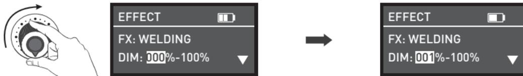
Rotate the knob to set the parameters of the corresponding options.
