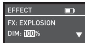
Press SWITCH button to select from DIM, CCT, G/M, SPD and DECAy.
