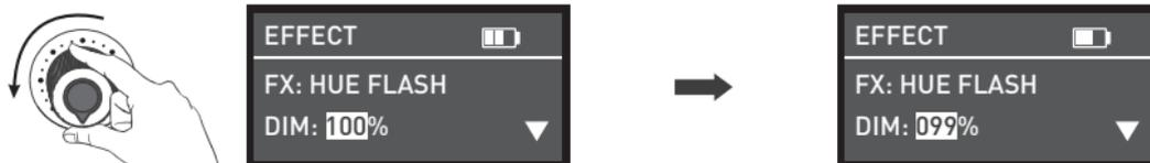
Rotate the knob to set the parameters of the corresponding options.
