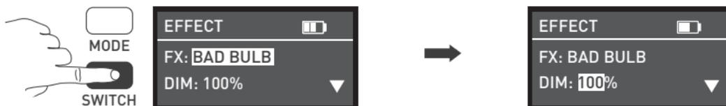
Press SWITCH button to select from DIM, CCT, G/M and SPD.
