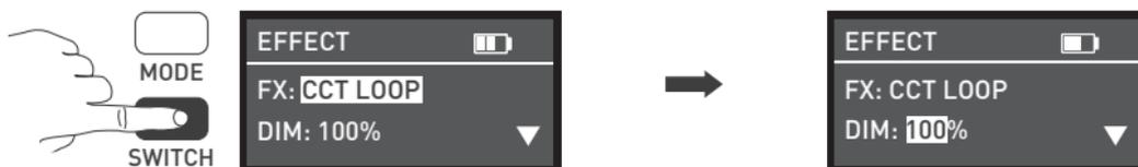
Press SWITCH button to select from DIM, CCT and SPD.
