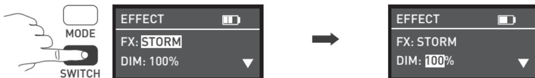
Press SWITCH button to select from DIM, CCT and INTVL.
