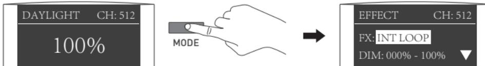
Press the MODE button to switch to the special effect interface.
