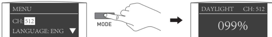
Press the MODE button, enter the daylight mode.
