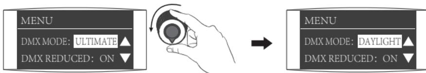
Rotate the left knob to select desired DMX mode.
