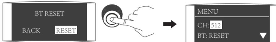
Press the "right knob" to confirm the reset and it will return to the menu after Bluetooth reset.
