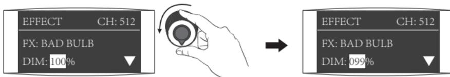
Rotate the "left knob" to set the corresponding parameters as required.
