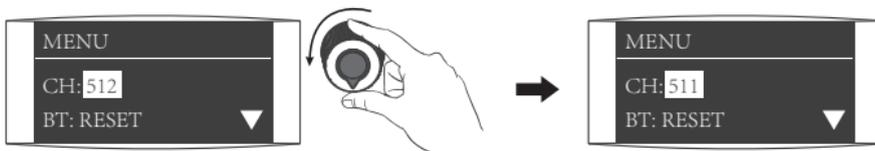
Rotate the "left knob" to set the channel.
