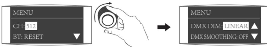
Rotate "right knob" to DMX DIM CURVE.
