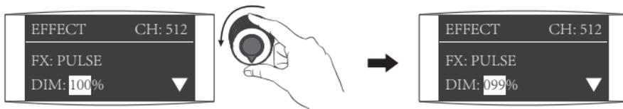
Rotate the "left knob" to set the corresponding parameters.
