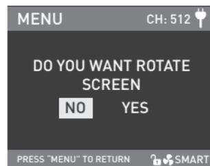
Rotate the "right knob" to ROTATE SCREEN, and press the "right knob" to enter the corresponding secondary menu.
