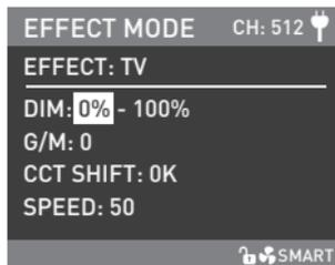
Rotate the "right knob" to select DIM, G/M, CCT SHIFT or SPEED.
