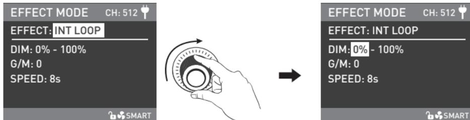
Rotate the "right knob" to select DIM, G/M or SPEED.
