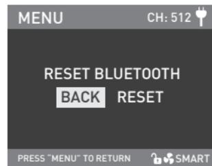
Rotate the "right knob" to RESET BLUETOOTH, and press the "right knob" to enter the corresponding tertiary menu.
