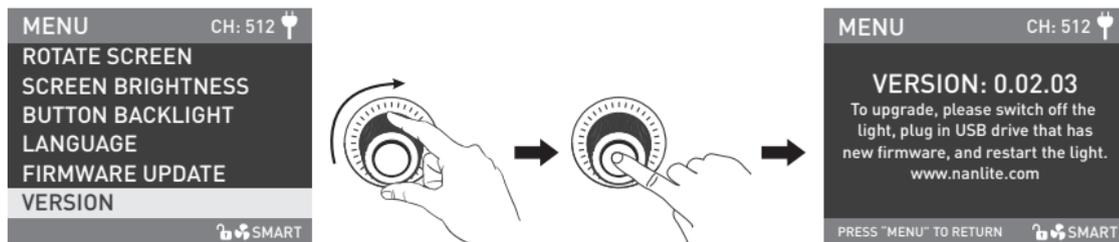
Rotate the "right knob" to VERSION, and press the "right knob" to check the current version.
