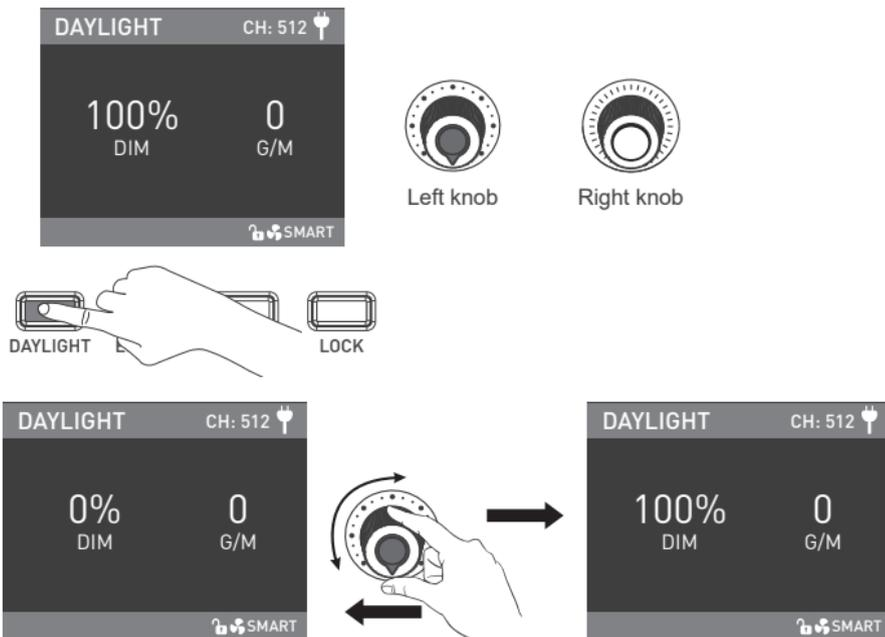
Rotate the "left knob", clockwise to increase brightness while counterclockwise to reduce the brightness. The screen shows the percentage of brightness, DIM range: 0%...100%.
