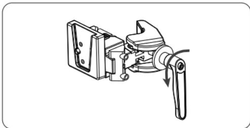
① Rotate the adjustable handle to release the clamp.
