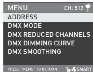
Rotate the "right knob" to ADDRESS/DMX, and press the "right knob" to enter the corresponding secondary menu.
