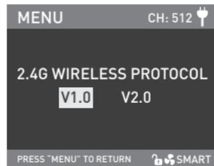
Rotate the "right knob" to WIRELESS PROTOCOL, and press the "right knob" to enter the corresponding tertiary menu.
