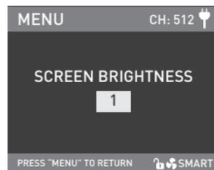
Rotate the "right knob" to SCREEN BRIGHTNESS, and press the "right knob" to enter the corresponding secondary menu.
