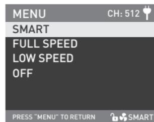
Rotate the "right knob" to FAN CONTROL, and press the "right knob" to enter the corresponding secondary menu.
