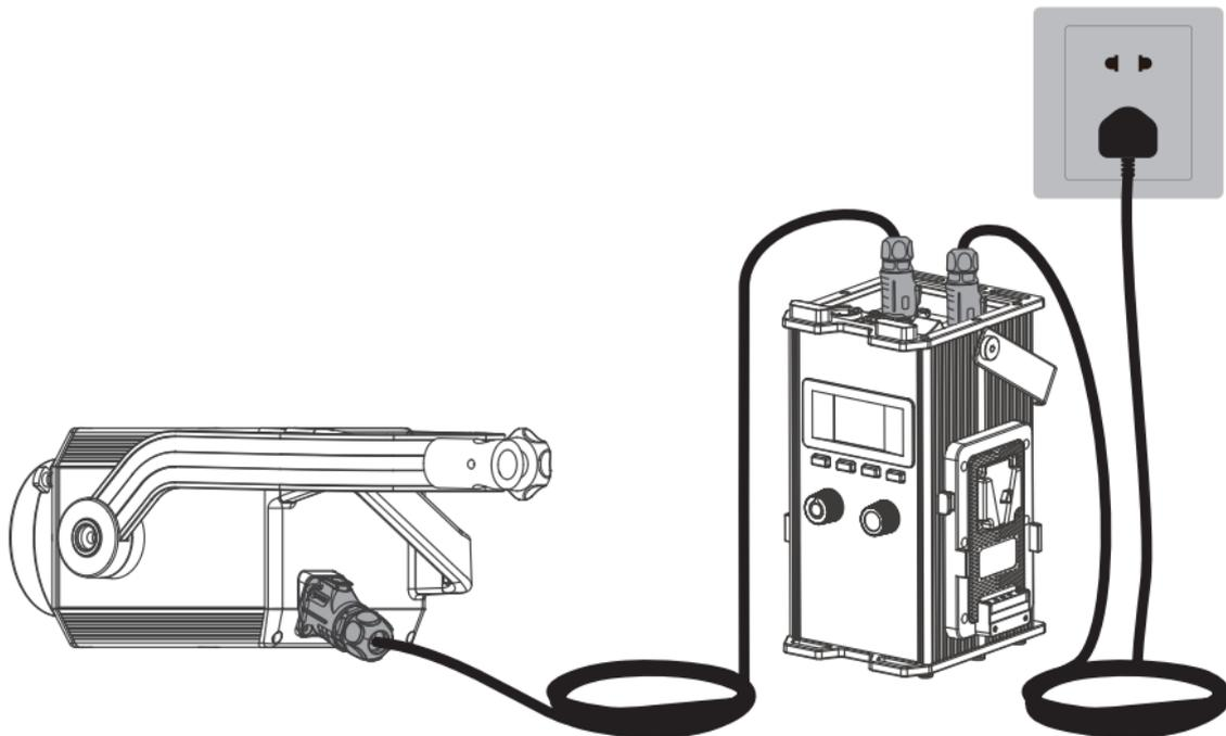
Note: ①When connecting the power supply, please make sure the power voltage are consistent with that indicated on the control unit.
