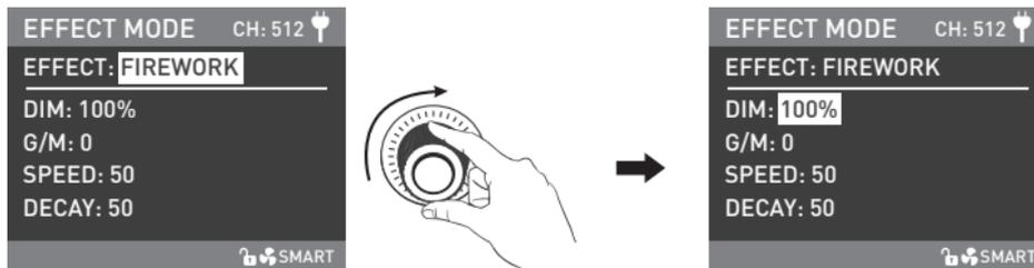
Rotate the "right knob" to select DIM, CCT, SPEED or DECAY.
