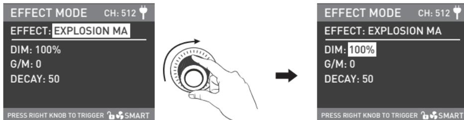
Rotate the "right knob" to select DIM, G/M or DECAY.
