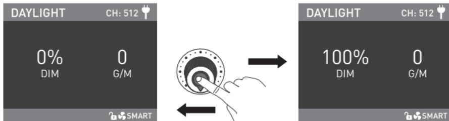
Press the "left knob" to turn off the fixture. Press again to restore the fixture to its previous state.
