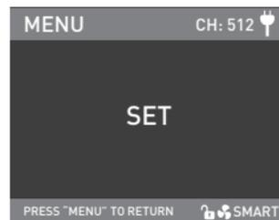
Rotate the "right knob" to select DAYLIGHT 8bit or ULTIMATE DMX 8bit, and press the "right knob" to set.
