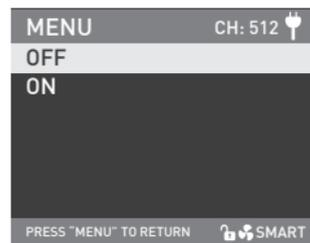
Rotate the "right knob" to DMX SMOOTHING, and press the "right knob" to enter the corresponding tertiary menu.
