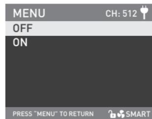
Rotate the "right knob" to DMX REDUCED CHANNELS, and press the "right knob" to enter the corresponding tertiary menu.
