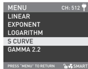
Rotate the "right knob" to DMX DIMMING CURVE, and press the "right knob" to enter the corresponding tertiary menu.
