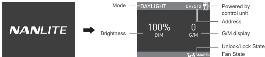
2. DAYLIGHT button: Press the DAYLIGHT button to enter the DAYLIGHT MODE.
