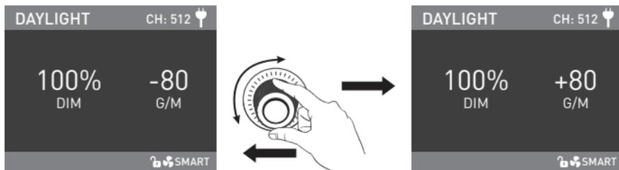
Rotate the "right knob" to set the corresponding parameters of G/M, the G/M range: -80...+80.
