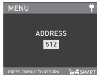
Rotate the "right knob" to ADDRESS, and press the "right knob" to enter the corresponding tertiary menu.
