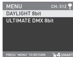
Rotate the "right knob" to DMX MODE, and press the "right knob" to enter the corresponding tertiary menu.
