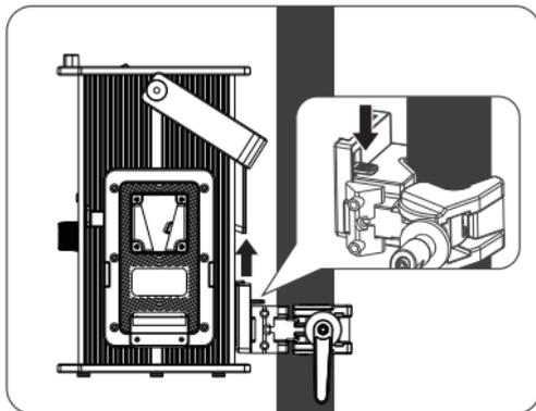
④ Press the lock catch on the clamp to remove the control unit from the light stand.
