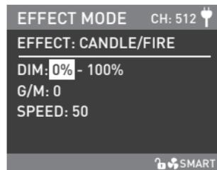
Rotate the "right knob" to select DIM, G/M or SPEED.
