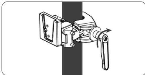
② Mount the quick release clamp on the light stand, then rotate the adjustable handle to tighten the clamp.
