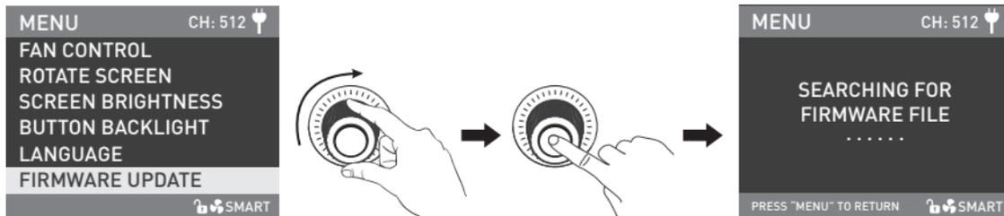
Rotate the "right knob" to FIRMWARE UPDATE, press the "right knob" to enter the interface to search for the firmware files.
