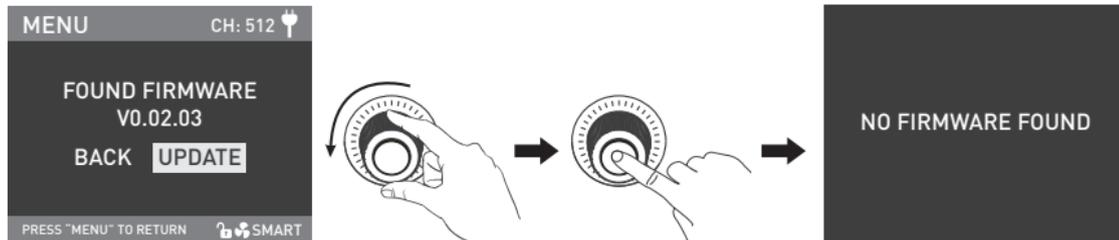
After finding the firmware file, enter the firmware update selection interface, rotate the "right knob" to select UPDATE, and press the "right knob" to make update. After update, the light fixture will automatically restart.
