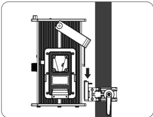
③ Align the quick release plate on the control unit with the quick release mount on the clamp to mount the control unit on to the clamp.
