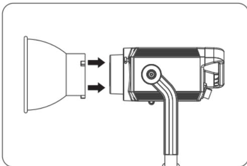
① When installing the reflector, align the reflector to the fixture's Bowens mount, rotate the reflector in the direction shown on the fixture until it clicks into place.
