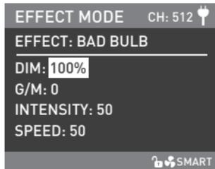
Rotate the "right knob" to select DIM, G/M, INTENSITY or SPEED.
