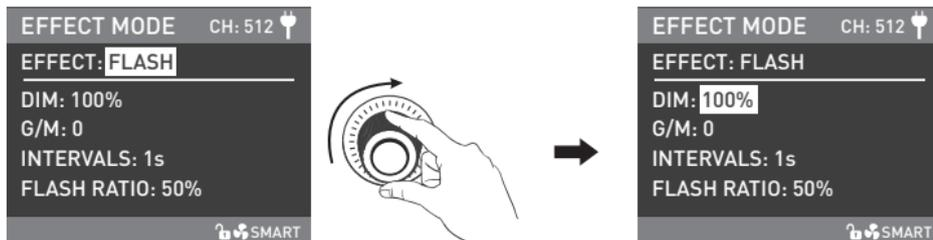
Rotate the "right knob" to select DIM, G/M, INTERVALS or FLASH RATIO.
