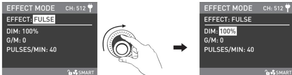
Rotate the "right knob" to select DIM, G/M or PULSES/MIN.
