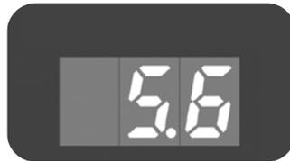
Push the **+** button to increase color temperature or push the **-** button to decrease it. If you keep pushed any of the buttons you will get a fast continuous variation. Every push on the buttons will increase or decrease the color temperature in increments of 100 Kelvin.
