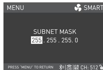
Rotate the right knob to SUBNET MASK, and press the right knob to enter the tertiary menu.
