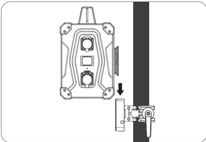
Align the quick release plate on the power supply with the quick release mount on the clamp, a click sound will be heard when the power supply is fastened in place.
