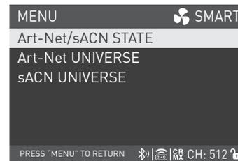
Rotate the right knob to Art-Net & sACN SETTINGS, and press the right knob to the secondary menu.
