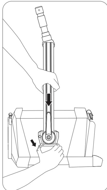
Firmly hold the yoke in place with one hand, and pull the quick release lever with the other hand to lock the plate.
