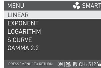
Rotate the right knob to DMX DIMMING CURVE, and press the right knob to enter the tertiary menu.
