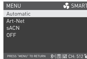
Rotate the right knob to Art-Net / sACN STATE, and press the right knob to the tertiary menu.
