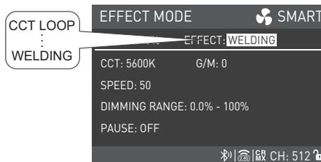
Rotate the middle knob to select the effect, which can be toggled in a loop.
