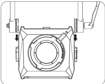
Align and insert the quick release plates to the mounts on both sides of the fixture.
