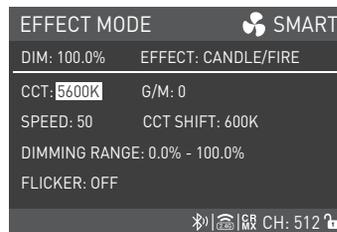
Rotate the right knob to select CCT, G/M, SPEED, CCT SHIFT, DIMMING RANGE or FLICKER.
