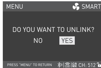
Rotate the right knob to UNLINK, and press the right knob to enter the next level menu.
