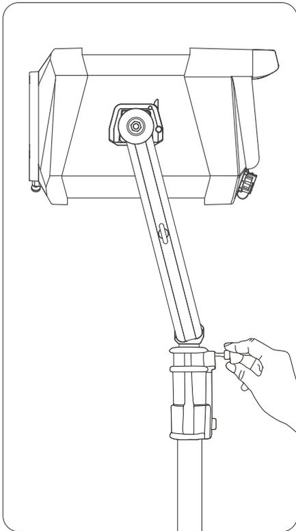
Mount the fixture on heavy-duty light stand and lock the fastening screws on the light stand.
