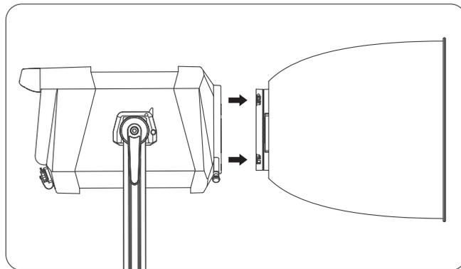
When removing the reflector, pull the lock catch of the mount, rotate anticlockwise the reflector and remove it.
