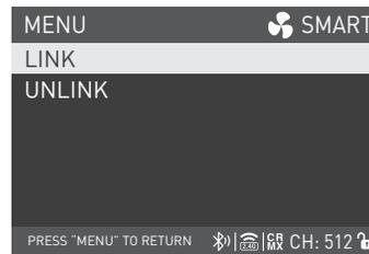
Rotate the right knob to LINK, and press the right knob to enter the next level menu.
