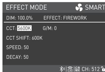
Rotate the right knob to select CCT, G/M, CCT SHIFT, SPEED or DECAY.
