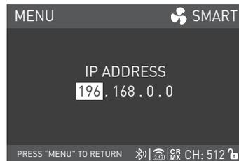
Rotate the right knob to IP ADDRESS, and press the right knob to enter the tertiary menu.
