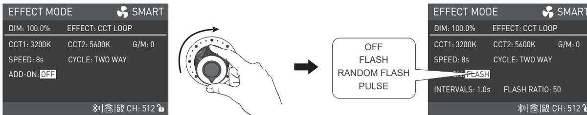
Rotate the middle knob to set the parameters.
