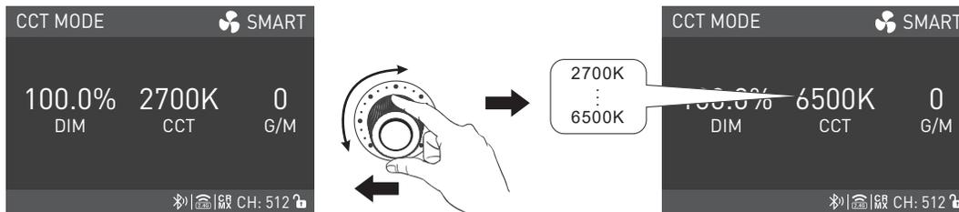
Note: In other modes, the CCT adjustment range is the same as in CCT mode. Press the right knob to promptly switch among 2700K, 3200K, 4300K, 5600K, 6500K, which can be toggled in a loop.
