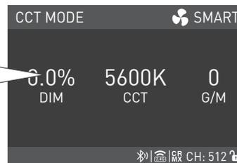
Note: In other modes, the brightness adjustment range is the same as in CCT mode. When the fixture function is unlock, in any mode, press the left knob, the light will be off, the brightness percentage on the screen will be 0.0%, press again, the fixture restores the previous state, press continuously to switch the light between on and off.
