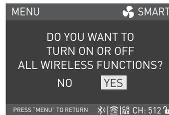
Rotate the right knob to ALL WIRELESS ON/OFF, and press the right knob to the tertiary menu.
