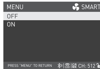
Rotate the right knob to LUMENRADIO ON/OFF, and press the right knob to enter the next level menu.
