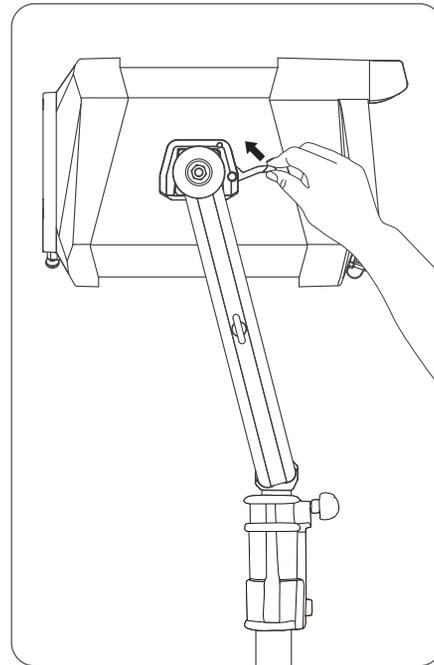
Pull the levers on both sides of the fixture to lock the quick release plate in place. The installation of the yoke is completed.
