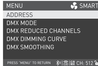
Rotate the right knob to ADDRESS/DMX, and press the right knob to enter the secondary menu.
