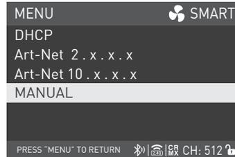
Rotate the right knob to NETWORK MODE, and press the right knob to enter the tertiary menu.
