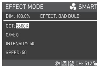
Rotate the right knob to select CCT, G/M, INTENSITY or SPEED.
