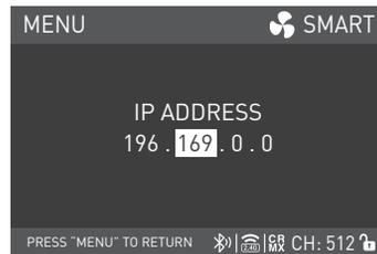
Rotate the right knob to the bytes, and rotate the middle knob to select the needed IP address.
