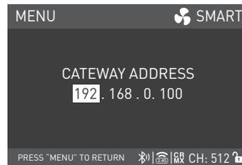
Rotate the right knob to GATEWAY ADDRESS, and press the right knob to enter the tertiary menu.
