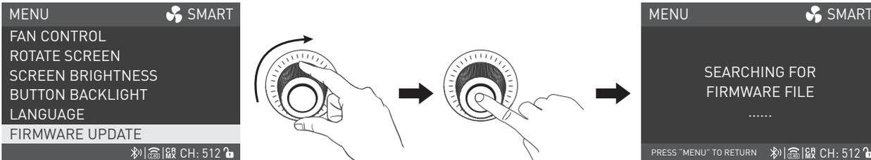
Rotate the right knob to FIRMWARE UPDATE, and press the right knob to enter the interface to search for the firmware files.
