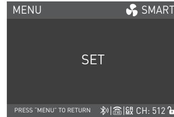
Rotate the right knob to select LINEAR, EXPONENT, LOGARITHM, S CURVE or GAMMA 2.2, and press the right knob to set.
