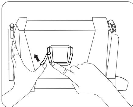
Press the quick release lever lock catch to release the lever, and push the lever aside.
