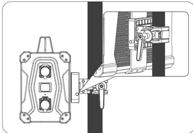
Press the lock catch on the clamp to remove the power supply from the light stand.
