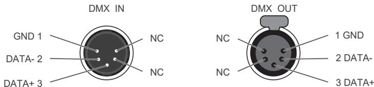
·5-pin shielded cable with a diameter not less than 0.3mm must be used for connection between light fixture and DMX/RDM console, or between light fixture and light fixture. XLR plug/socket and the cable should be connected as picture above.
