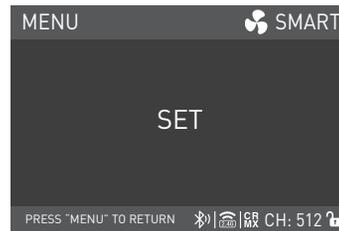
Rotate the right knob to select CCT 8bit, CCT 16bit or ULTIMATE DMX 8bit, and press the right knob to set.
