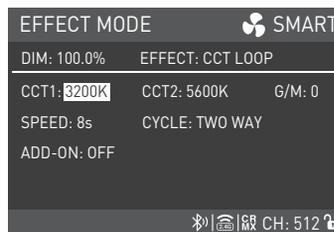
Rotate the right knob to select CCT 1 , CCT 2, G/M, SPEED, CYCLE or ADD-ON.
