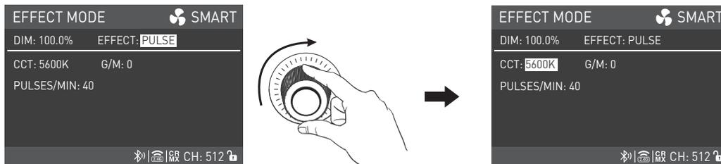
Rotate the right knob to select CCT, G/M or PULSES/MIN.
