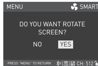
Rotate the right knob to the ROTATE SCREEN, and press the right knob to enter the secondary menu.
