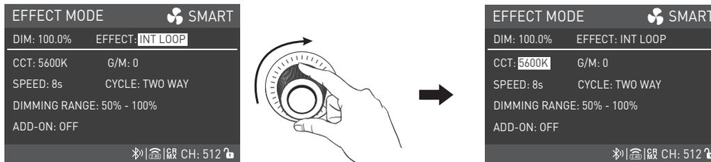
Rotate the right knob to select CCT, G/M, SPEED, CYCLE, DIMMING RANGE or ADD-ON.
