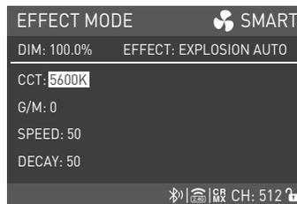
Rotate the right knob to select CCT, G/M, SPEED or DECAY.
