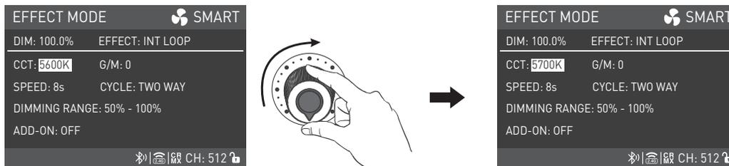
Rotate the middle knob to set the parameters.
