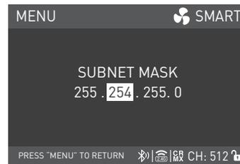
Rotate the right knob to the subnet, and rotate the middle knob to select the needed subnet mask.
