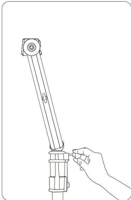
Mount the yoke on heavy-duty light stand and lock the fastening screws on the light stand.
