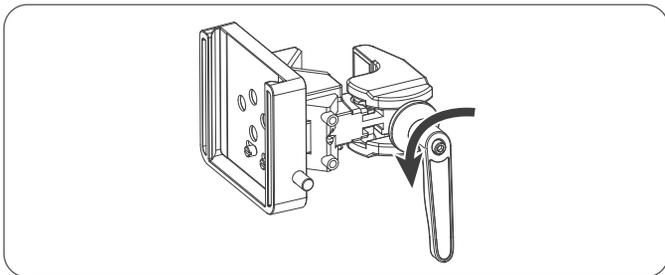
Rotate the adjustable handle to release the clamp.
