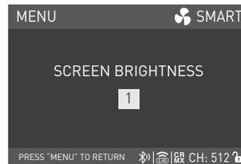
Rotate the right knob to SCREEN BRIGHTNESS, and press the right knob to enter the secondary menu.
