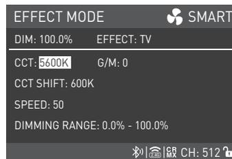
Rotate the right knob to select CCT, G/M, CCT SHIFT (range: 0K-3000K), SPEED (range: 1-100) or DIMMING RANGE.
