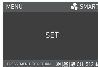
Rotate the right knob to select speed: SMART, FULL SPEED, LOW SPEED or OFF, and press the right knob to set.
