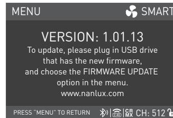
Rotate the right knob to VERSION, and press the right knob to check the current version.
