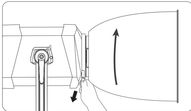
When installing the reflector, align the reflector to the NL mount on the fixture, rotate clockwise the reflector to fasten it on the fixture.
