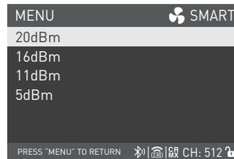
Rotate the right knob to RF OUTPUT POWER, and press the right knob to enter the next level menu.
