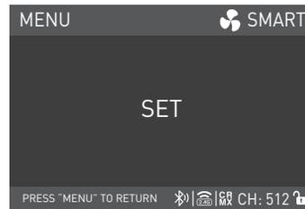
Rotate the right knob to select ON or OFF, and press the right knob to set. The 2.4G wireless control is available when the 2.4G is set to be on.
