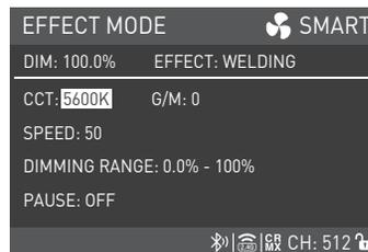
Rotate the right knob to select CCT, G/M, SPEED, DIMMING RANGE or PAUSE.
