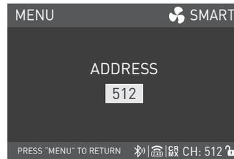
Rotate the right knob to ADDRESS, and press the right knob to enter the tertiary menu.
