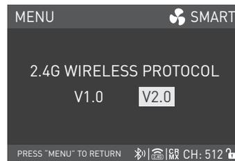
Rotate the right knob to WIRELESS PROTOCOL, and press the right knob to enter the next level menu.
