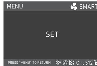
Rotate the right knob to select MAX OUTPUT or CONSTANT OUTPUT, and press the right knob to set.
