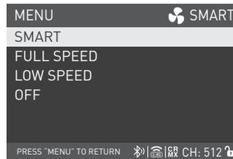
Rotate the right knob to FAN CONTROL, and press the right knob to enter the secondary menu.
