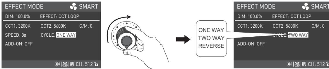
Rotate the middle knob to set the parameters.
