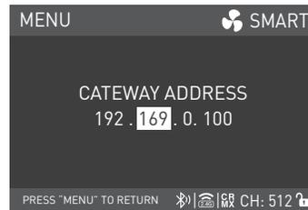
Rotate the right knob to the bytes, and rotate the middle knob to select the needed gateway address.
