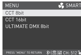
Rotate the right knob to DMX MODE and press the right knob to enter the tertiary menu.
