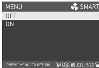
Rotate the right knob to 2.4G ON/OFF, and press the right knob to enter the next level menu.
