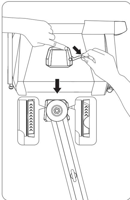
Press the quick release lever lock catch and push the lever aside, align and insert the quick-release plate mounts to the plates of the yoke.
