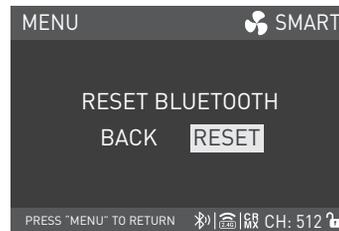
Rotate the right knob to RESET BLUETOOTH, and press the right knob to enter the next level menu.
