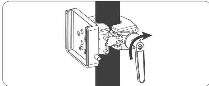
Mount the quick release clamp on the light stand, then rotate the adjustable handle to tighten the clamp.
