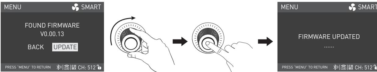
After the firmware file is found, enter the firmware update interface, rotate the right knob to select UPDATE, and press the right knob to make update.
